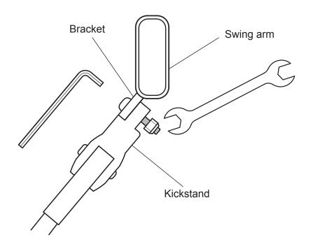
To install the kickstand follow the above illustration using a 3mm Allen key and 8mm wrench. Place the kickstand under the swing arm bracket and tighten the included bolts and nut to 75-90Lbs/ln.
