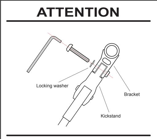
To install the kickstand follow the above illustration using a 3mm Allen key. Place the kickstand inside the bracket and tighten the included bolt and locking washer to 75-90Lbs/ln.
