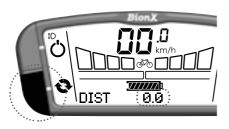
To reset the cycle computer functions
